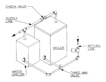
Figure 3.2: Parallel Hook-Up with Water Chiller
